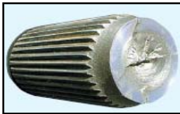
Failed Semi-truck Axle shaft
