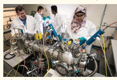
Graduate students in Ram Gupta's lab work on combined "sputtering and thermal evaporator," equipment that helps them develop incredibly thin layers of material.
