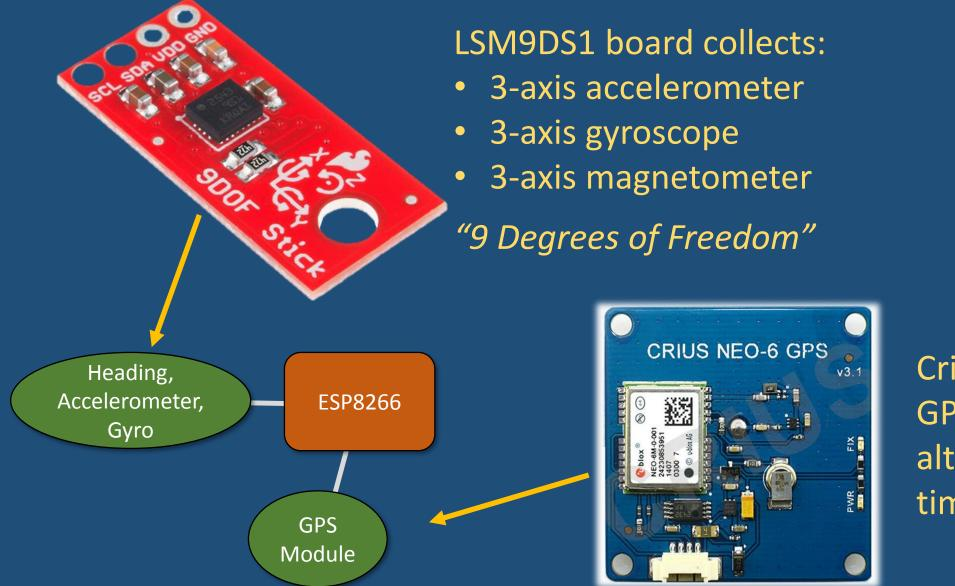
Crius NEO-6 provides GPS coordinates and altitude plus accurate timing
