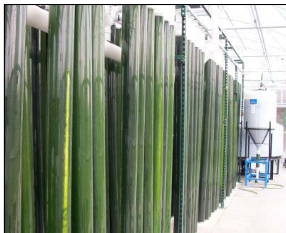
a scale up photobioreactor of over 13,000 gallons of algae, currently in use at CAER
